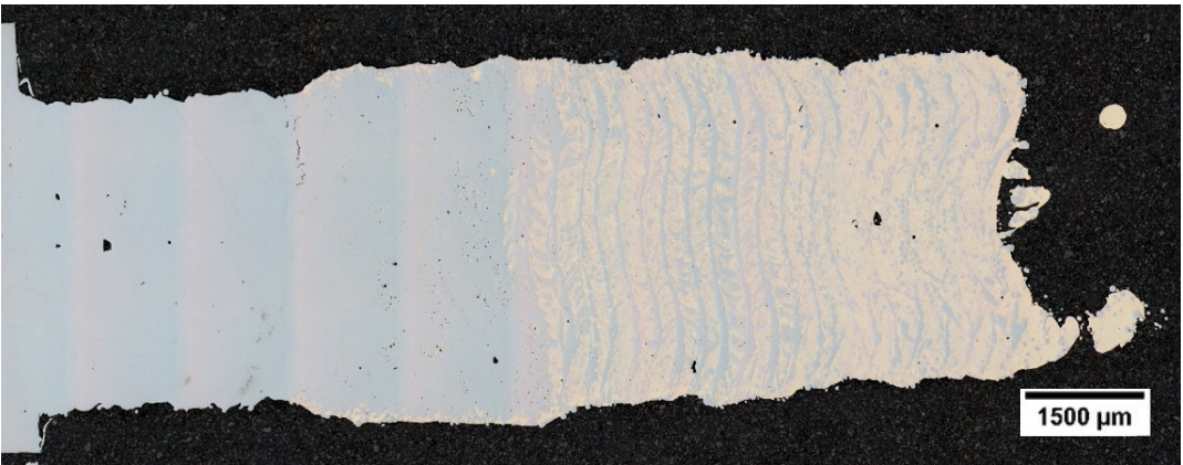
An H13-Cu FGM sample manufactured using LDED. (Subproject 1.2.2 | Craig, Owen. "MATERIAL CHARACTERIZATION OF DIRECTED ENERGY DEPOSITION OF H13 TOOL STEEL AND FUNCTIONALLY GRADED H13-COPPER." (2022).)
